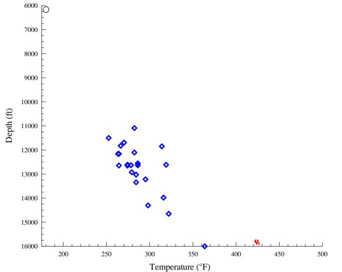
Precision temperature log and BHT data for areas in the Texas and Louisiana. All three areas are situated in the high gradients areas paralleling the Gulf Coast. The existence of temperatures in excess of 250 °F by 9,000-12,000 ft suggest favorable conditions for future geothermal development.
